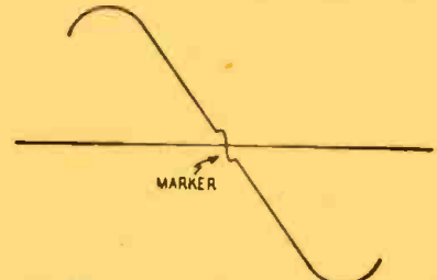
Fig. 8—Marker signals identify frequencies.
