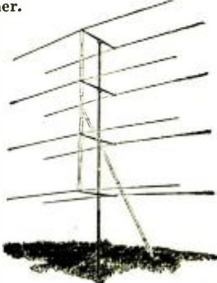
Fig. 6—A sensitive and directional antenna.
