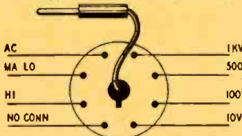
Fig. 5—Pin connections for range selector.
